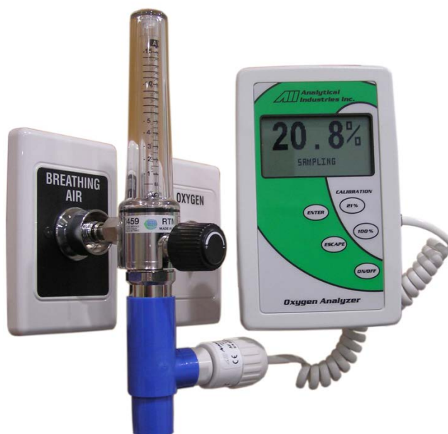
Figure 1. Example of gas analyser for testing gas identity at the terminal unit
