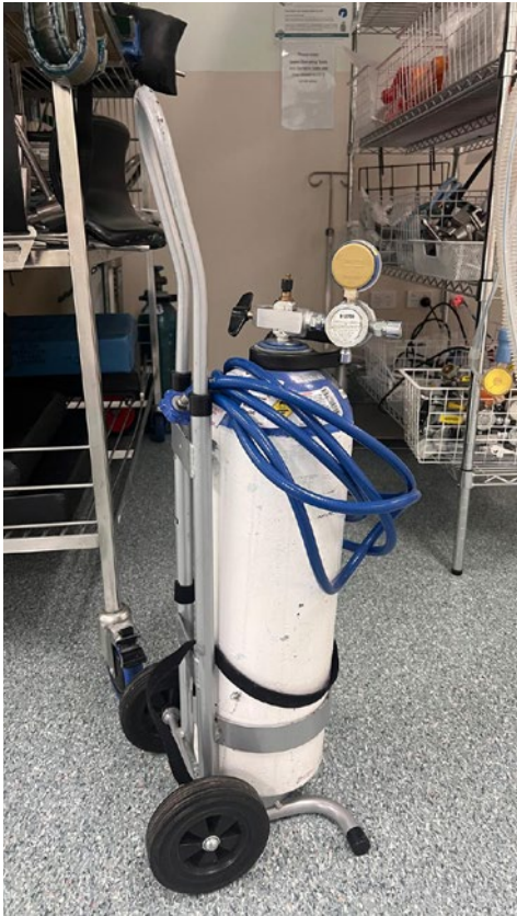
ABOVE FROM LEFT Decommissioned N 2 O wall outlet. Portable nitrous trolley system for PRN connection.
